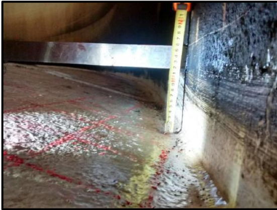
Dimensional do recalque
