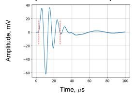
Echo pulse duration: 26.8  $\mu$ s AFC frequency maximum  $f_p$ : 112.3 kHz Lower AFC frequency  $f_l$ : 73.1 kHz Upper AFC frequency  $f_u$ : 138.9 kHz
