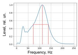
Operating frequency  $f_c$ : 106.0 kHz AFC maximum  $S_{rel}$ : -50.9 dB Absolute transmission bandwidth P: 62.6 kHz Relative transmission bandwidth  $B_w$ : 61.1 %
