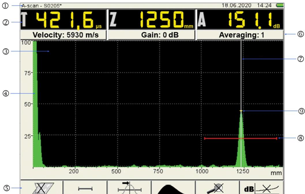
**Figure 15: Screen layout of the A-SCAN mode**
