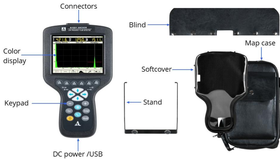
Figure 1: A1221 ANCHOR hardware components
