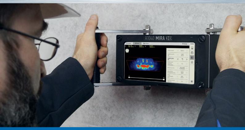
• <u>True3D® Tomography</u> - three-dimensional FMC / TFM in each instrument position in real time
